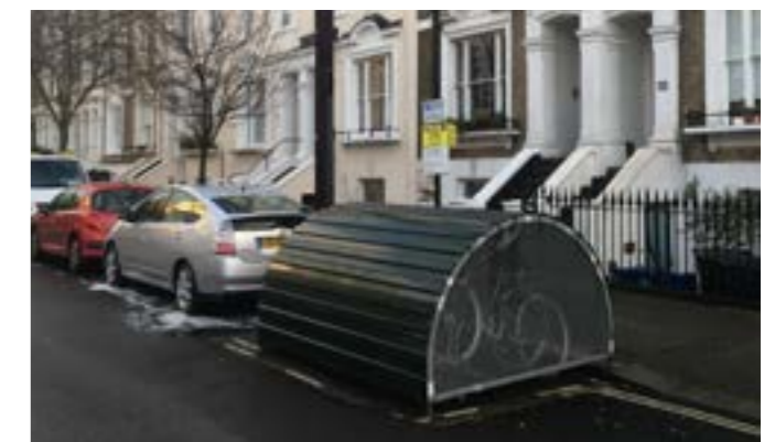
Good practice precedent: A cycle hanger In the space to park one car, a cycle hanger can provide secure and convenient storage of six bicycles, encouraging uptake of cycling.
