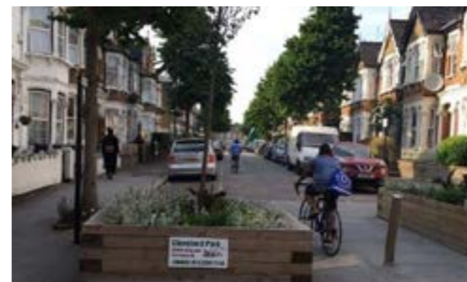
Good practice precedent: A quietway and modal filter This quietway provides a pleasant environment for people walking and cycling. The modal filter allows bicycles and pedestrians through while stopping cars.
