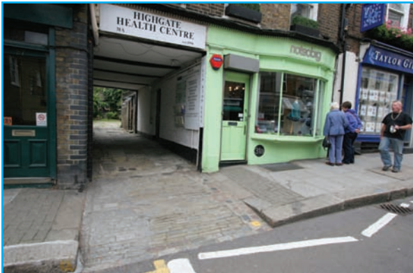
Footway crossover access to commercial premises
