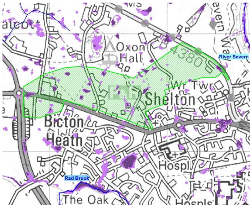
Figure 3-4 – FMfSW results for the 0.5% AEP rainfall event for the Western SUE © Crown copyright and database right 2012 Ordnance Survey licence number 100049049
